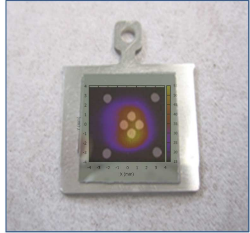
Fig. 1. Typical beam profile, obtained on analyzing images from a beam viewer placed behind the irradiation mask for 3 keV \text{Na}^+ ions, superimposed on an image of an Omicron-style sample holder showing the four centrally located irradiated devices and the four pristine devices at the corners. The color scale indicates intensity of an illuminated pixel in the beam viewer image used to obtain the profile. For this measurement, the beam current measured through an aperture of \sim 6 \text{ mm} diameter was 12.33 nA.
